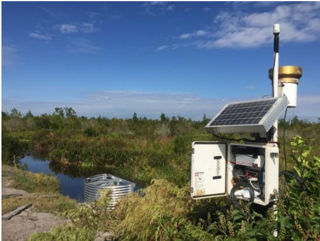
Water level monitoring station showing a weir on the left, and the datalogger on the right, including solar panel, rain gauge and antenna. The water level transducer is submerged in the ditch (not seen in the image). Photo by Archbold Biological Station.
