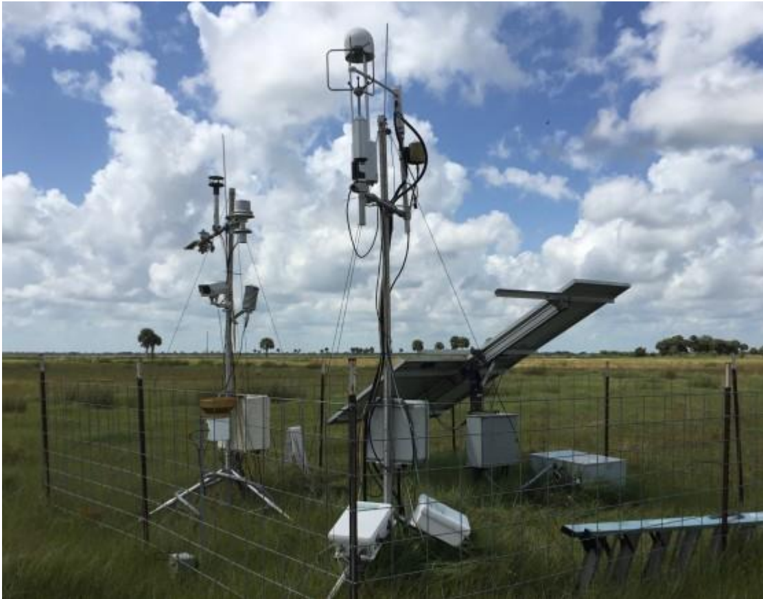
A weather station (left) and Eddy Flux tower (right) at MAERC used to measure uptake and emissions of greenhouse gases by soils, cows, and vegetation. Photo by Archbold Biological Station.
